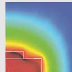
**Thermal** provides the temperature maps obtained by the balance between the Fourier heat transport and the Joule heat. The deep integration with **Drift-Diffusion** makes **Thermal** a powerful tool for thermal analysis of devices
