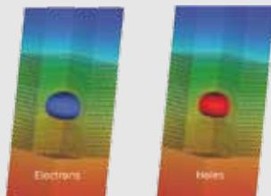
Transport of electrons and holes is calculated based on the **Drift-Diffusion** approximation. Mechanical, thermal and quantization effects can be included self-consistently by coupling to the **Elasticity**, **Thermal** and
