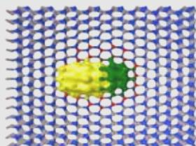
Atomistic models for quantum calculation of electronic and optical properties of nanostructures with Empirical Tight Binding (ETB). Combined with a built-in atomistic generator and a structure relaxation tool based on Valence Force Field (VFF), it
